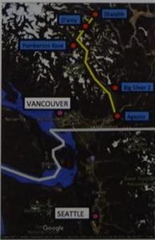
Fig. 2. Approximate location of the 360 kV transmission line (yellow), weather stations used surrounding the line (red).
