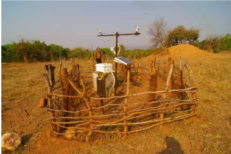
Rain gauge; Installed 16 in each site
